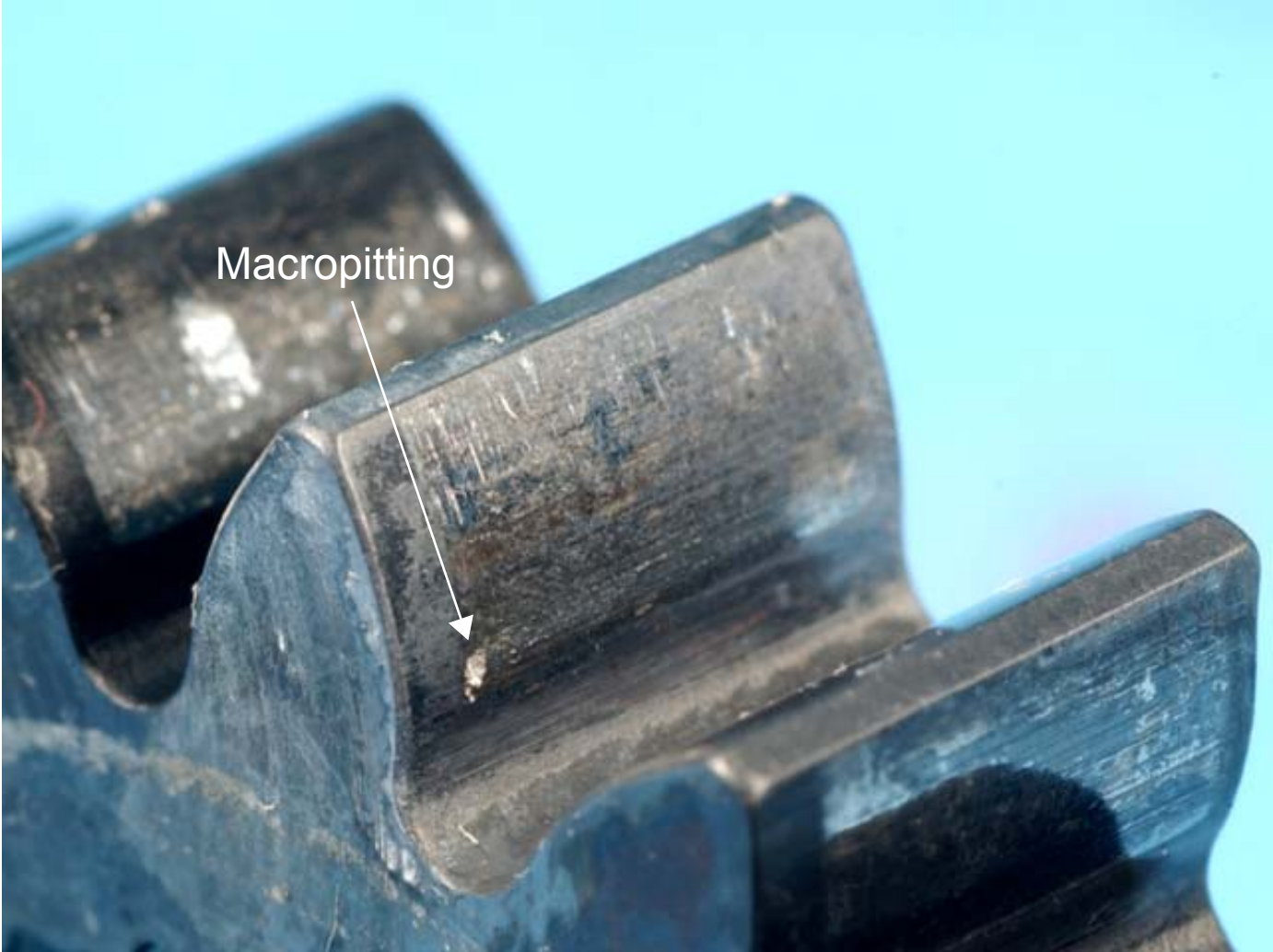
No wear on tooth surface. Initial light macropitting.
